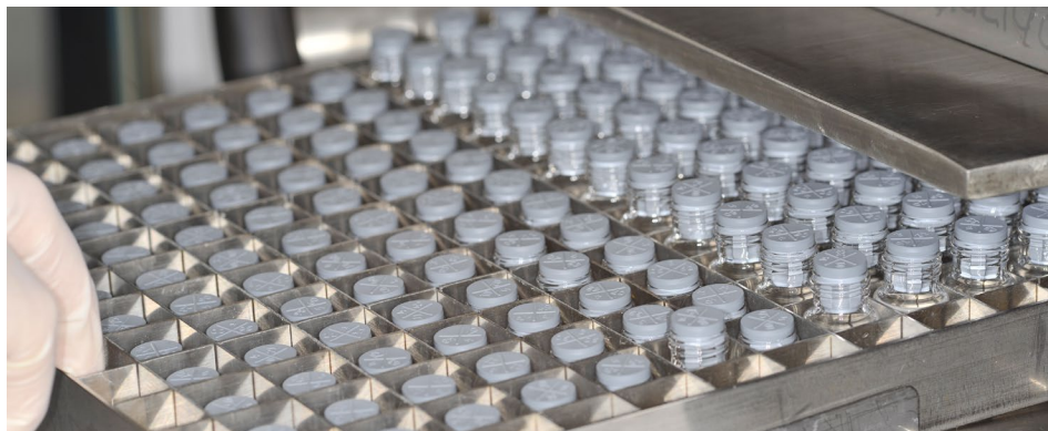
Glass vials are ideal for reagent manufacture: glass is impervious to both oxygen and moisture
